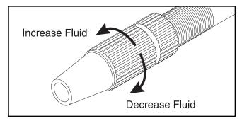
Figure 3. Adjusting flow.
